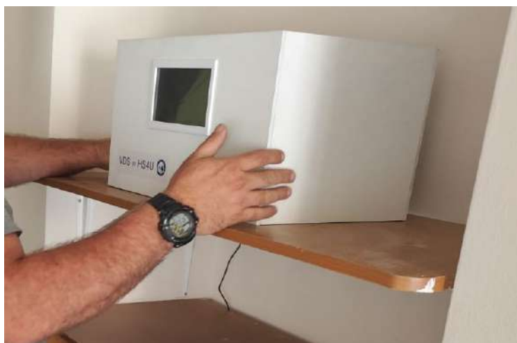
Figure 6: VDS device installed in the entertainment room. The device was strategically positioned to sample air from vents, thus enabling effective real-time monitoring of airborne pathogens within the enclosed space.
